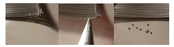
In addition, should the edges of the belt obstruct the entry of the spiral conjunction, they will have to be opened manually and any links obstructing the spiral removed.
