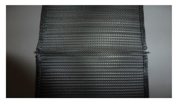
After the belt has been in use for a week or two, it will settle naturally, becoming about 40/50 cm longer. It will then be necessary to shorten it, by cutting off the excess material.
