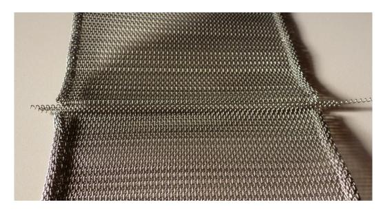
6. Use scissors/shears to cut the protruding part of the spirals, or bend them upwards as if to form the continuation of the edge.
